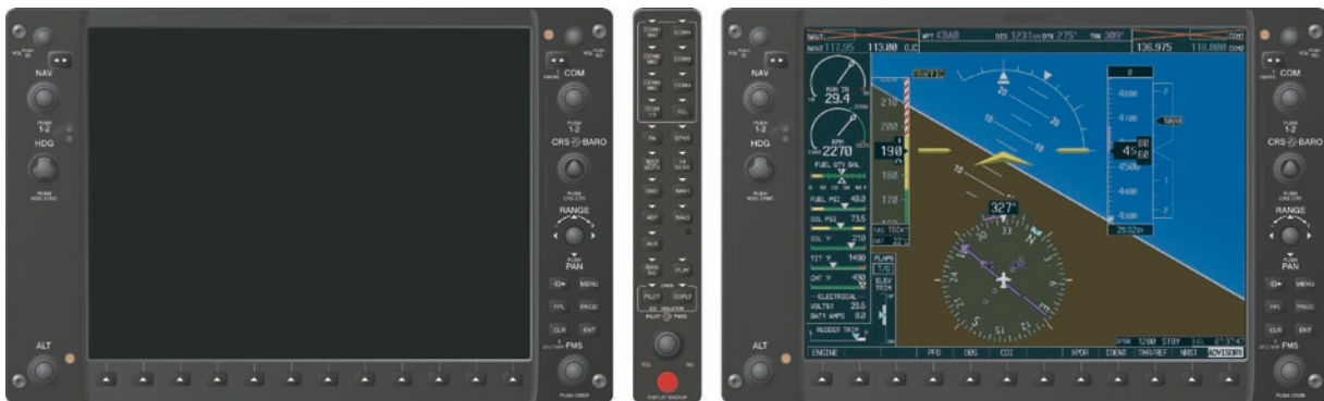
Figure 1-4 G1000 Reversionary Mode: Failed PFD
