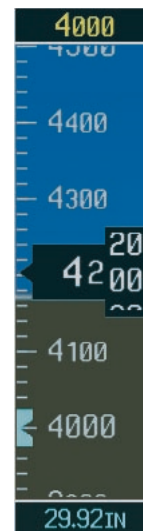
Figure 2-13 Altimeter within 200 ft. of Reference Altitude
