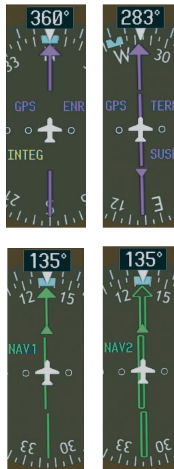
Figure 2-25 GPS INTEG, GPS SUSP, NAV1 and NAV2
