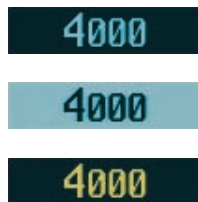
Figure 2-11 Colors Associated with the Altitude Alerter
