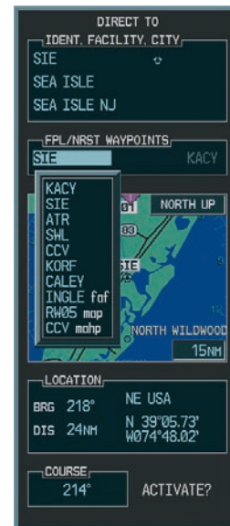
Figure 4-19 Flight Plan Waypoint Direct-to
